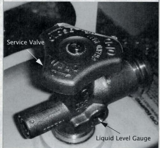
Figure 5-21 Fixed Maximum Liquid Level Gauge on DOT/TC cylinder
