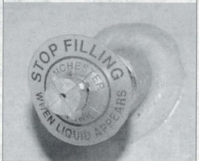
Figure 5-22 Fixed Maximum Liquid Level Gauge on ASME Tank
