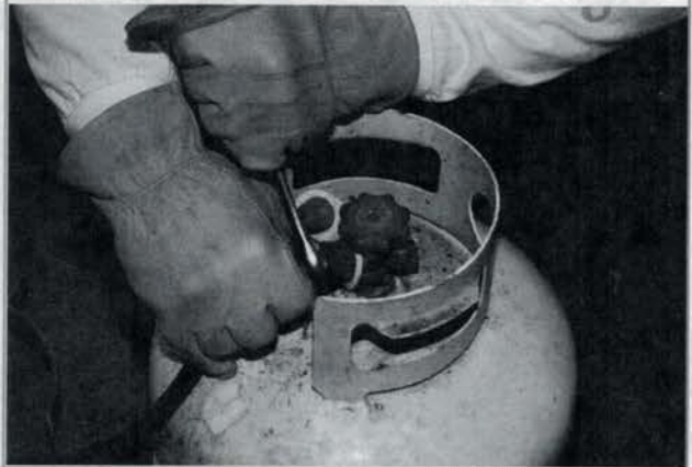
Figure 5-5 Tighten POL with Wrench (Pre-2002)
